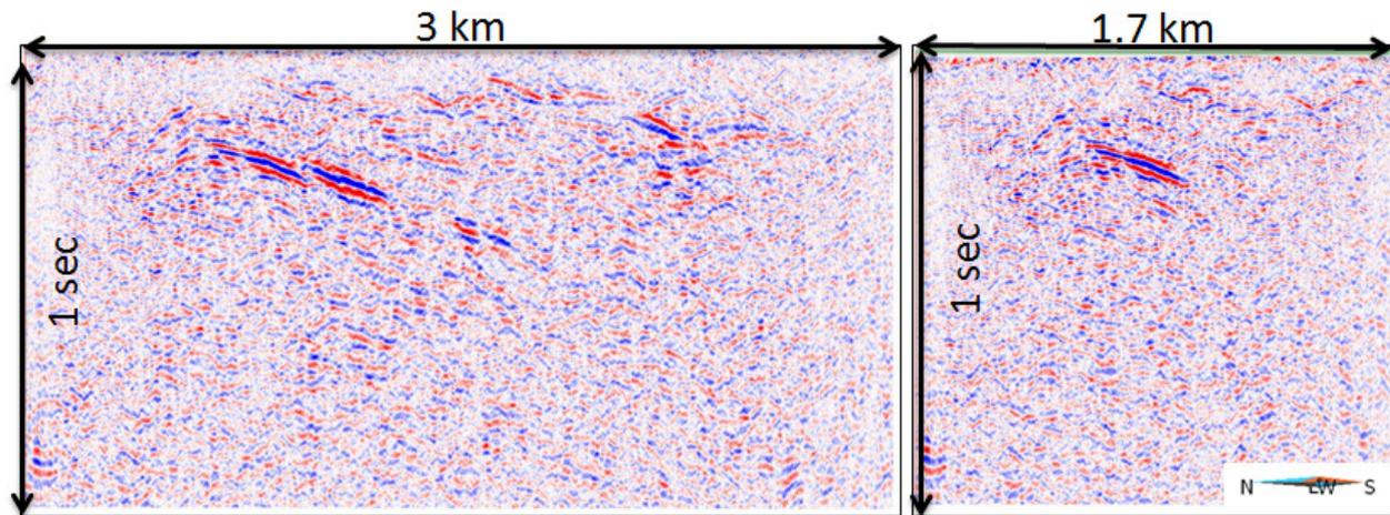
**Figure 1** Stack with full 2D geometry (left) and stack using line length and maximum offset as in the 3D survey (right) in time. The down-dip component of the high amplitude reflection is only imaged with the full 2D geometry.
