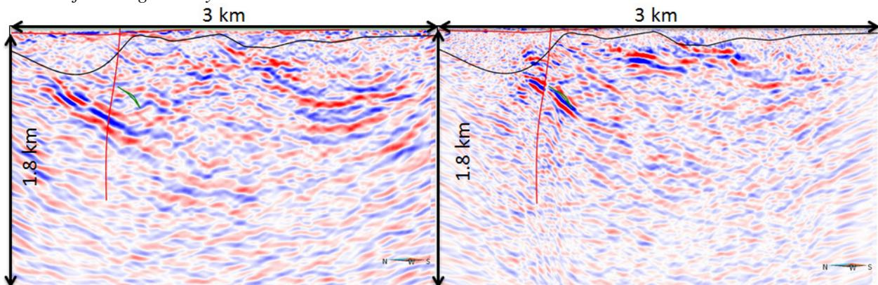
**Figure 2** 2D migrated sections using the standard (left) and tomography driven approach (right) in depth. Sub-vertical red line and dipping green line represent a major fault and massive sulphide respectively. Both are accurately imaged using the tomography driven approach.
