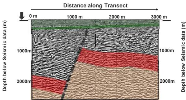
**Figure 4: Seismic transect targeting a large north south fault in the northern Gngangara mound, Perth Basin, WA. Carefully targeted seismic provides a clear hydrogeological framework for a fault and upper angular unconformity surface. The stacked seismic data is presented as a cosine of phase attribute.**
