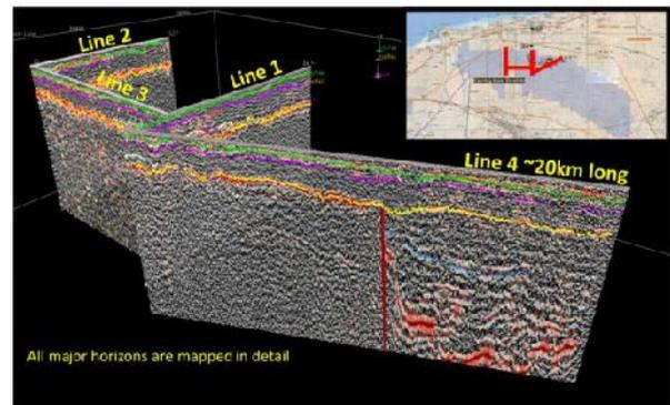
**Figure 2:3D volume of all the 2D seismic transects over the Canning Basin. The aquifer can be traced across the large scale basinal fault located along line 4. This figure illustrates the value tracing aquifers in 2D transects over a large 3D area. Figure from FMG, 2012.**
