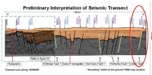
**Figure 1: Seismic reflection transect with schematic interpretation overlay spanning across the Allanooka region of the Perth Basin. Notice the large scale structural fault illustrated by the red circle that acts as boundary extent for the basin (the image is taken from Gavin, 2010). Lisa's interpretation shows the boundaries and lateral geometry of the aquifer are directly related to faulting.**
