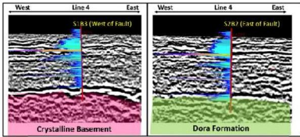
**Figure 4: seismic reflection transect of Line 4 with gamma log mapped over the seismic. “The seismic appears to have mapped significant units including a basal sand unit within the Wallal Sandstone immediately above crystalline basement (~195 to ~240m). The yellow and green spikes in the gamma log are high gamma and relate to clay/claystone horizons” (FMG, 2012). This gamma log information can be extrapolated across the length of the seismic.**
