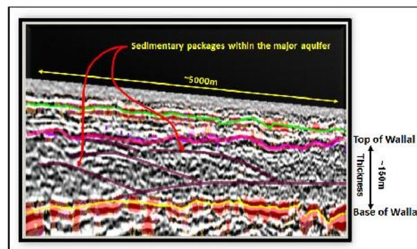
**Figure 3: Transect along a canning basin 2D seismic line. Notice how well distinct packages of sedimentary rock are expressed within Wallal aquifer target. The seismic survey was specifically designed to have high resolution in the depth range 0 to 250m. Figure from FMG 2012.**
